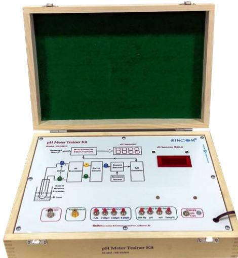
**SINCOM SE-1045 pH Meter Demonstrator** is a comprehensive trainer for studying the measurement of pH value of a given liquid using PH sensors. This trainer is equipped with advanced features such as a Digital LED Display, pH sensor, Temperature sensor. The trainer also features an Auto Calibration Inputs, selection of different measuring inputs like pH, Temperature & mV of a given liquid under test.
