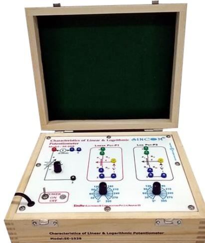
**SINCOM SE-1028 Characteristics of Potentiometer & its loading effect** is a versatile trainer designed for studying the characteristics & loading effect of potentiometers. It allows users to analyze the behaviour of these potentiometers when subjected to variable DC input voltage and multiple resistors. The potentiometer features an on-board 0-300° marked shaft angle dial, providing precise control and measurement for both types of potentiometers.
