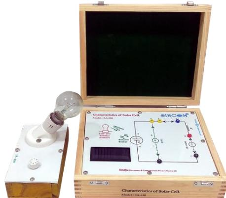
**SINCOM SE-1101 Solar Cell Characteristics** is remarkable trainer for examining the operation, characteristics and parameters of a solar cell in varying conditions with the facility to apply artificial variable intensity light source.
