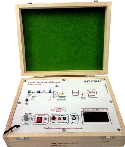
**SINCOM SE-1020 Open Loop Control System** is a highly adaptable and comprehensive trainer that is specifically designed for studying the impact of an open loop control system on the temperature of a heater load. This system includes an RTD temperature sensor, OP-AMP based circuitry, a digital temperature indicator, and an electrical heater load. Additionally, it offers the convenience of setting the reference temperature input, allowing for precise control and analysis.
