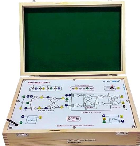
**SINCOM SC-907/SC-310 Flip-Flop Trainer** is a self contained trainer to verify the operation & truth table of RS,JK,JKMS,D & T Flip-Flops using logic gates and ICs, with the facility to apply logic Inputs, logic output Indicator, Mono clock Pulse generator and DC Power Supply.
