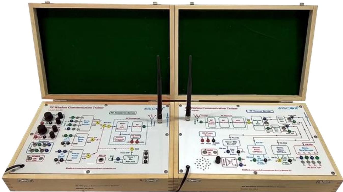
**SINCOM SA-941 RF Wireless Communication Trainer** serves as an extensive training system for the study of the Transmission and Reception of Analog and Digital Data Input using ASK RF wireless communication link. This trainer features Analog Audio Inputs , Voice/MIC audio input, 4 bit Parallel Digital Data Input and Serial Data Input, Speaker and TX RX Antennas. It includes the capability to study the signal and voltage analysis of RF communication link.
