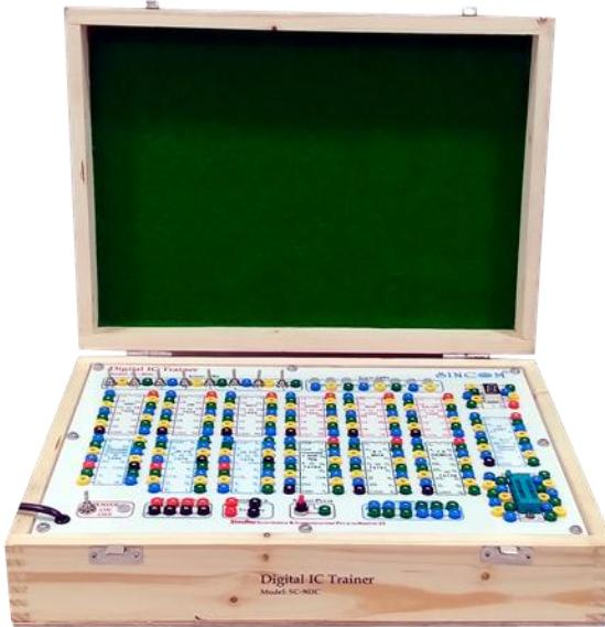
**SINCOM SC-903 Digital IC Trainer** is a versatile self contained trainer to understand various experiments using TTL Digital ICs. This trainer offers the capability to verify the operation & truth table of Logic gates AND,OR,NOT,NAND,NOR,EX-OR, JK Flip-Flops, Universal Shift Register, Decade Counter, 8:1 Multiplexer, 1:8 Demultiplexer, Seven Segment Decoder, Code converters, Adder-Subtractors and their combinational circuits.
