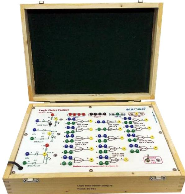
**SINCOM SC-901 Logic Gates Trainer** is a self contained trainer to verify the operation and truth table of AND,NAND,OR,NOR,NOT,EX-OR,EX-NOR logic gates using ICs and the basic logic gates AND,OR,NOT using Diode Transistors. This is an essential trainer for understanding and experimenting with logic gates in a simple way.
