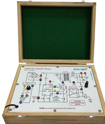
**SINCOM SB-127 SMPS for Mobile Phone** is a remarkable very useful simply designed trainer to study the operation, line and load regulation characteristics of a Switching Mode Power supply (SMPS) for Mobile Phone application in a simple experimental way. The Trainer is without meters and has the facility to connect the external analog or digital Voltmeter and Ammeter in the circuit.
