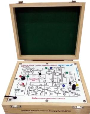
**SINCOM SB-121 Switching Mode Power Supply (SMPS) Trainer** is a remarkable very useful simply designed trainer to study the concept, operation, line and load regulation characteristics of a Switching Mode Power supply (SMPS) in a simple experimental way. The Trainer is without meters and has the facility to connect the external analog or digital Voltmeter and Ammeter in the circuit.
