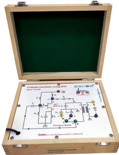
**SINCOM SE-143 Colpitts Oscillator using JFET** is a useful trainer to study the concept and operation of Colpitts Oscillator with LC positive feedback to generate RF Output Frequency using JFET with facility to select multiple radio frequencies in a simple experimental way.
