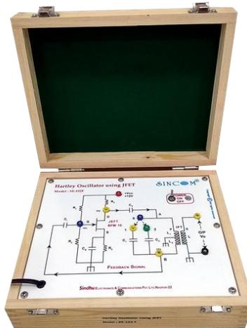
**SINCOM SE-142 Hartley Oscillator using JFET** is a useful trainer to study the concept and operation of Hartley Oscillator with LC positive feedback to generate RF Output Frequency using JFET with facility to select multiple radio frequencies in a simple experimental way.
