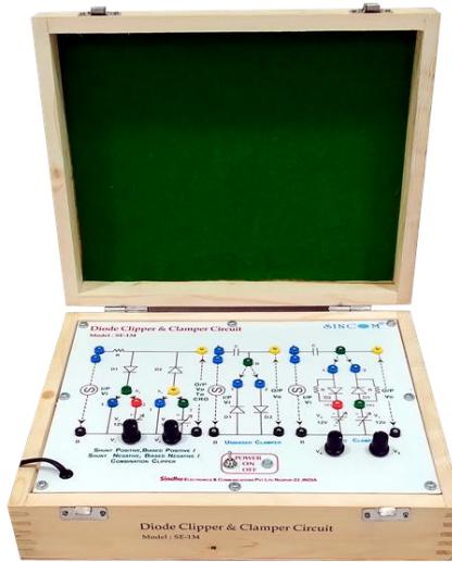
**SINCOM SE-134 Diode Clippers and Clampers circuit** is a remarkable All-In-One useful trainer with PN Junction Diode, resistors, capacitors and variable positive/negative bias voltage to provide Diode shunt positive, negative, combinational with & without bias clippers and Diode Positive/Negative clampers with & without bias, with facility to vary the clipping and clamping level in a simple experimental way.
