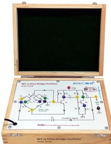
**SINCOM SE-109 Wein Bridge Oscillator** is a useful trainer to study the concept and operation of Wein Bridge Oscillator with RC lead-lag positive feedback to generate AF Output Frequency using BJT with facility to select multiple audio frequencies in a simple experimental way.
