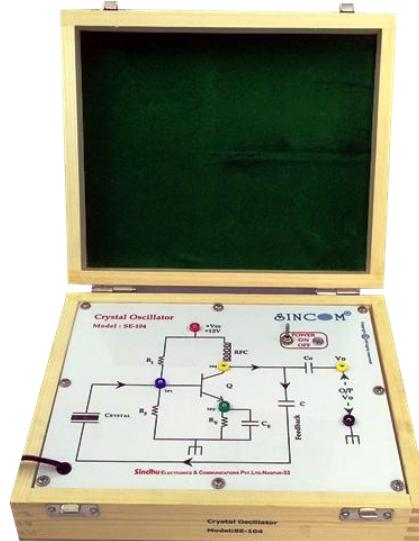
**SINCOM SE-104 Crystal Oscillator** is a useful trainer to study the concept and operation of Crystal Oscillator with Crystal positive feedback to generate RF Output Frequency using BJT in a simple experimental way.
