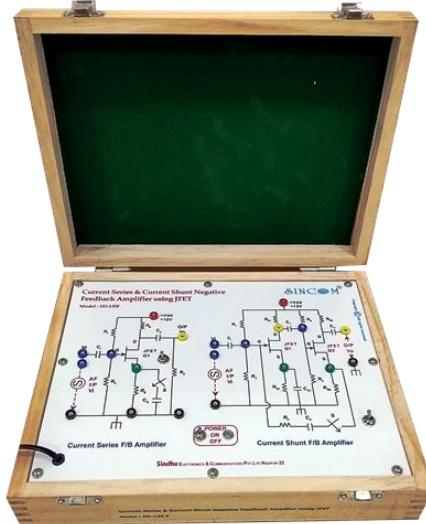
**SINCOM SD-150 Current Series and Current Shunt Negative Feedback Amplifier using JFET** is a Two-In-One remarkable simply designed trainer for the purpose to study the concept, operation, Frequency response and determine the Bandwidth, Voltage gain and other parameters of a Current Series and Current Shunt negative feedback Amplifier using JFET in a simple experimental way.
