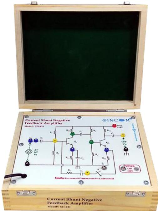
**SINCOM SD-131 Current Shunt Negative Feedback Amplifier using BJT** is a simply designed trainer for the purpose to study the concept, operation, Frequency response and determine the Bandwidth, Voltage gain and other parameters of a Current Shunt negative feedback Amplifier in a simple experimental way.
