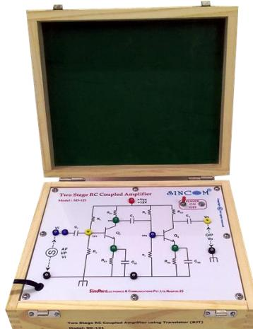
**SINCOM SD-121 Two Stage RC Coupled Amplifier using Transistor** is very useful simply designed trainer to study the concept, operation, Frequency response and determine the Bandwidth, over all Voltage gain and other parameters of a BJT Two stage RC coupled Amplifier in a simple experimental way.
