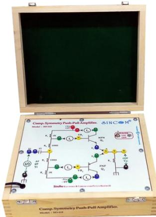
**SINCOM SD-112 Complementary Symmetry Push Pull Amplifier** is simply designed trainer for the purpose to study the concept, operation, Frequency response and determine the Bandwidth, Voltage gain and other parameters of a complementary symmetry Class-AB Push Pull Amplifier in a simple experimental way.
