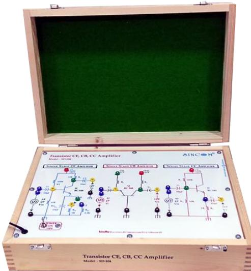
**SINCOM SD-104 Transistor Amplifier (Single Stage CE,CB,CC)** is All-In-One simply designed trainer for the purpose to study the concept, operation, Frequency response and determine the Bandwidth, Voltage gain and other parameters of BJT as Single Stage CE,CB,CC Amplifier with a gain control in a simple experimental way.
