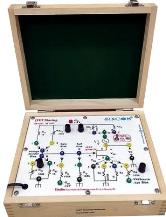
**SINCOM SC-107 JFET Biasing Trainer** is a **All-In-One** simply designed trainer for the purpose to study N-Channel JFET Gate Bias, Self Bias, Voltage Divider Bias, Source Bias methods and determine the various operational parameters with a wide range of components bank in a simple experimental way.
