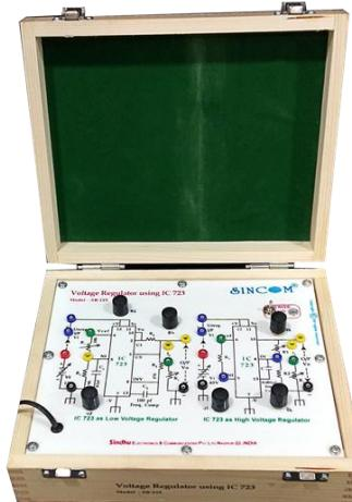
**SINCOM SB-115 IC723 as Positive Low and High Voltage Regulator** is a Two-In-One simply designed trainer very useful to study the operation, line and load regulation characteristics of IC723 as Positive Low and High Voltage Regulator with variable load in a simple experimental way. The trainer is without meters and has the facility to connect the external analog or digital Voltmeter and Ammeter in the circuit.
