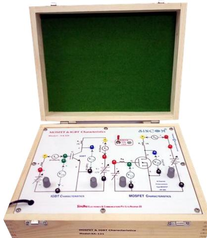
**SINCOM SA-121 MOSFET & IGBT Characteristics** is useful to study V-I characteristics of MOSFET and N-Channel IGBT. The power MOSFET and IGBT are mainly used in switching circuits and power electronics applications. The trainer is simply designed to plot its characteristics and determine the various operational parameters in a simple experimental way. The trainer is without meters and has the facility to connect the external analog or digital voltmeter and ammeter in the circuit.
