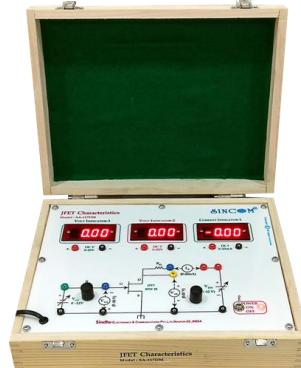
**SINCOM SA-117DM JFET Characteristics** with Digital meters is comprehensive remarkable trainer is useful to study Drain and Transfer characteristics of JFET. The JFET is widely used as a switching and an amplification device in many electronics circuits. The trainer is simply designed to plot its characteristics and determine the various operational parameters in a simple experimental way. The trainer is equipped with on board Digital voltmeter and Digital Ammeter.
