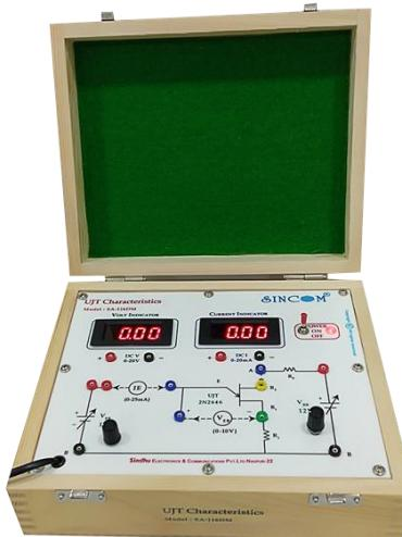
**SINCOM SA-116DM Uni-Junction Transistor (UJT) Characteristics** with Digital meters is comprehensive remarkable trainer is useful to study V-I characteristics of UJT. The UJT are widely used in Pulse, Switching, Timing, Sensing, Thyristor Phase control and voltage detector circuit. The trainer is simply designed to plot its characteristics and determine the various operational parameters in a simple experimental way. The trainer is equipped with on board Digital voltmeter and Digital Ammeter.
