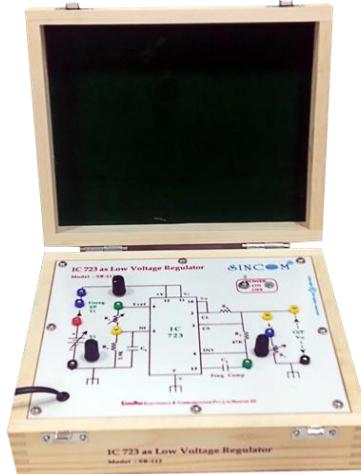
**SINCOM SB-112 IC723 as Positive Low Voltage Regulator** is very useful simply designed trainer to study the operation, line and load regulation characteristics of IC723 as Positive Low Voltage Regulator with variable load in a simple experimental way. The trainer is without meters and has the facility to connect the external analog or digital Voltmeter and Ammeter in the circuit.
