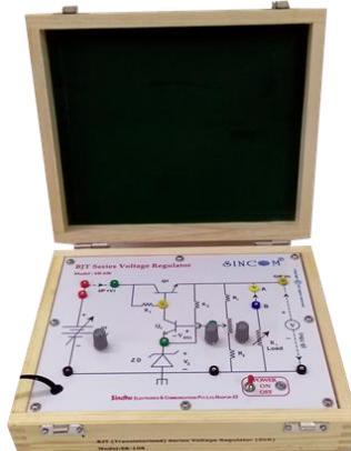
**SINCOM SB-108 BJT (Transistorized) Series Voltage Regulator** is very useful simply designed trainer to study the operation, line and load regulation characteristics of BJT Series Voltage Regulator with variable load in a simple experimental way. The trainer is without meters and has the facility to connect the external analog or digital Voltmeter and Ammeter in the circuit.
