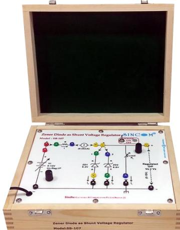
**SINCOM SB-107 Zener Diode as Shunt Voltage Regulator** is very useful simply designed trainer to study the operation, line and load regulation characteristics of Zener Diode as Shunt voltage Regulator with variable load in a simple experimental way. The trainer is without meters and has the facility to connect the external analog or digital Voltmeter and Ammeter in the circuit.
