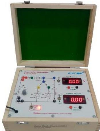
**SINCOM SA-102DM Zener Diode Characteristics** with digital meters is self contained trainer which is very useful to study the V-I characteristics different Zener Diodes which are widely used in various common need voltage stabilization circuits. The trainer is simply designed to plot the zener characteristics and determine the zener voltage under test in a simple experimental way. The trainer is equipped with on board Digital voltmeter and Digital Ammeter.
